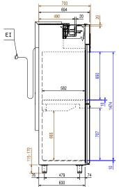
Electrical inlet (power) ΕI Refrigerant Inlet Refrigerant Outlet RO
